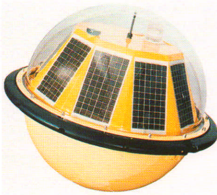
Figure 1.21 Solar-powered directional wave buoy (which in use is moored to the sea-bed). The buoy contains sensors that measure roll, pitch and yaw, as well as wave displacement, velocity and acceleration.
