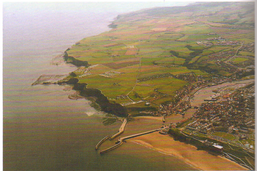
Figure 5.16 (a) The components of a coastal sediment budget. (b) Whitby harbour and mouth of the River Esk. The harbour blocks the south-eastward longshore drift and little sediment is deposited along the shore beyond.
