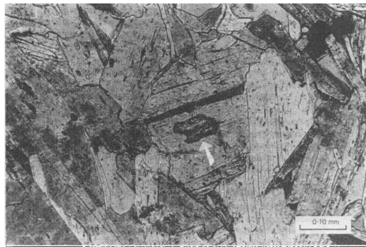
Fig. 6.5 Photomicrographs of metamorphic textures described in the text. a ) Granoblastic polygonal texture of quartz in kyanite quartzite. Kofi Mountain, north-east Tanzania, courtesy of R.A. Cliff. b ) Decussate texture of interlocking micas (primarily muscovite). The high relief grain (arrowed) is a relic inclusion of staurolite in muscovite. Pelitic schist from the sillimanite-muscovite zone, Connemara, Ireland.
