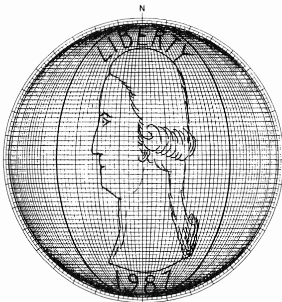
Figure 15-29. The principle behind De Paor's method. Coin can be made to appear circular by tilting the page away from you.
